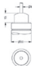
Cable outlet with PVC-cable (IP 67) 2
